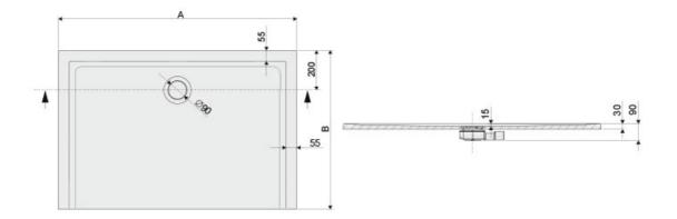
Basic dimensions: 700x800 mm Depth: 15 mm A dimension: 800 mm B dimension: 700 mm
